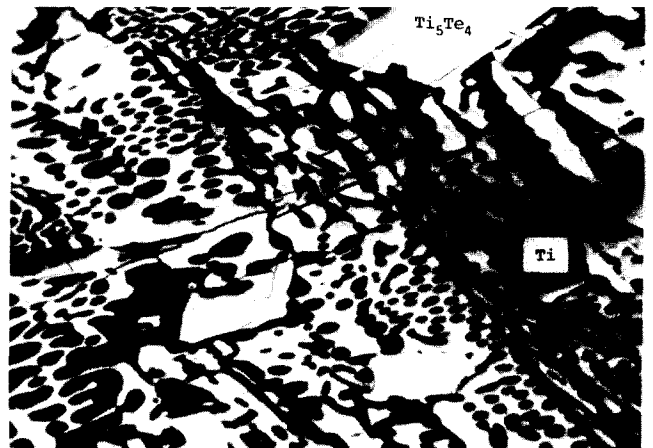
Fig. 9. Micrograph of a DTA sample with 33 at.% Te, solidified from 1330 °C, demonstrating the eutectic reaction L = \beta\text{-Ti} + \beta\text{-Ti}_5\text{Te}_4 with \text{Ti}_5\text{Te}_4 primary crystals (backscattered-electron image). The dark Ti regions consist of (Ti) and a eutectoid structure, which is not visible with this contrast setting.
